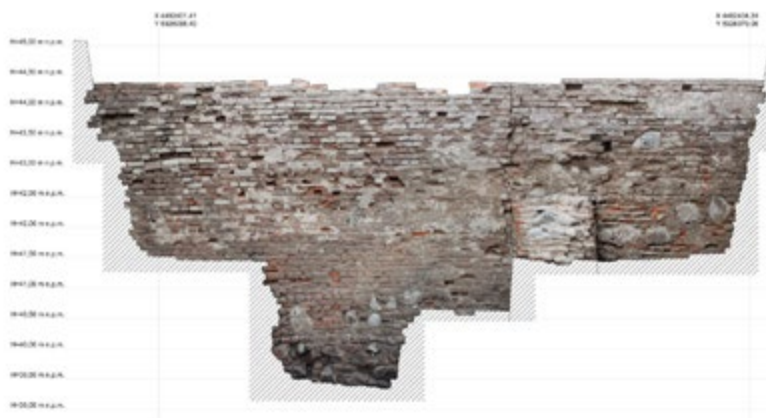
Figure 3 – Results of photogrammetry of the face of the wall at Pasłęk (done by R. Solecki).
