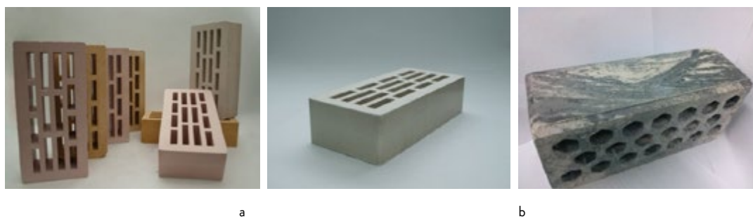
Figure 3 – Bricks of carbonate hardening from the pilot batch: a – with rectangular slit-like voids; b – dyed in imitation of marble in the mass with voids in the form of honeycomb.
