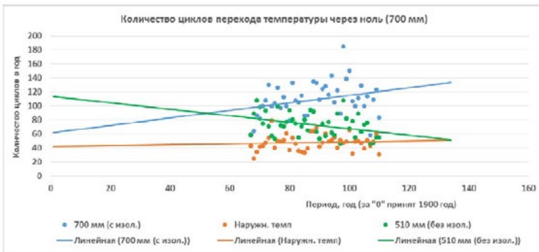
Figure 6 — Graphs of intensity of temperature of the year (Ni) for exterior brick walls 700 mm with and without insulation.
