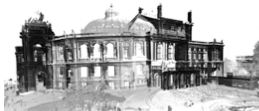
Figure 4 - Point clouds in the Cyclone program
