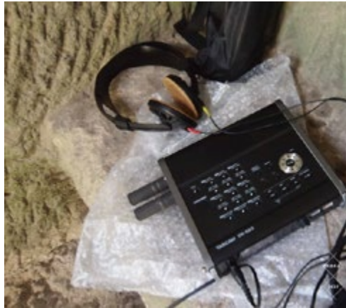
Figure 3 – The digital recorder Tascam DR-680 placed inside the structure carved in the rock behind the pyramid with the microphones inserted in the body of the device.
